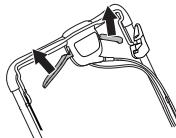
When the drive starts feeling slow you need to adjust the clutch wire. Finely adjust the wire using the adjuster screw.
